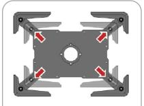
Adjust tablet shell by sliding the grips in the direction indicated by the arrows to fit your tablet.
