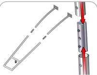
Connect bottom tubes following the labels by matching number to number. Slide joiner into tubing so hex screw sits in hole on tubinger.
