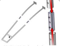
CONTINUED: Tighten the hex screw so the joiner seperates and tightens against the inside of the tubing, locking the joiner & tubing together.
